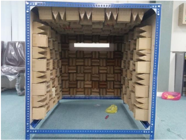
Fig. 6 - Installation wedge pattern
