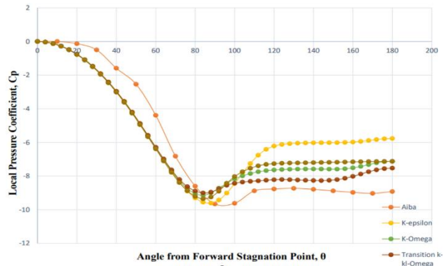
Fig. 1 – Local pressure coefficient, C p vs angle from forward stagnation point, θ
