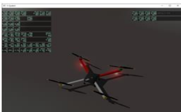
Fig. 9 - Quadcopter model in X-Plane
