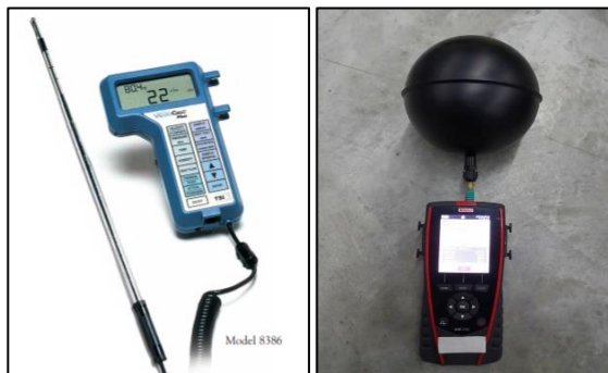
Fig. 2 - Velocicalc Plus Multi-parameter Ventilation Meter 8386 (left) and KIMO AMI 310 with black globe thermometer (right).
